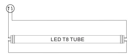
Note B: Please operate fixture it works with single tube follow above wiring scheme which insert tube nondirectional.
