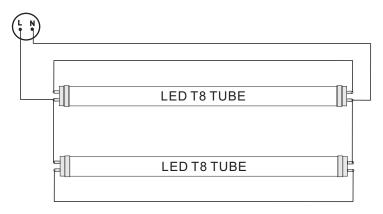
Note C: Please operate fixture it works with double tube follow above wiring scheme that insert tube nondirectional.
